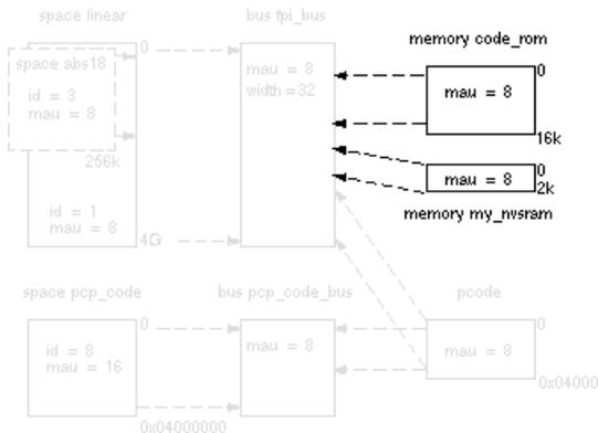
Suppose your embedded system has 16 kB of external ROM, named `code_rom` and 2 kB of external NVRAM, named `my_nvsram`. Both memories are connected to the bus `fpi_bus`. In LSL this looks like:
