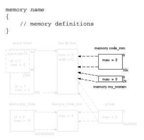
Suppose your embedded system has 16 kB of external ROM, named code\_rom and 2 kB of external NVRAM, named my\_nvsram. Both memories are connected to the bus fpi\_bus. In LSL this looks like:
