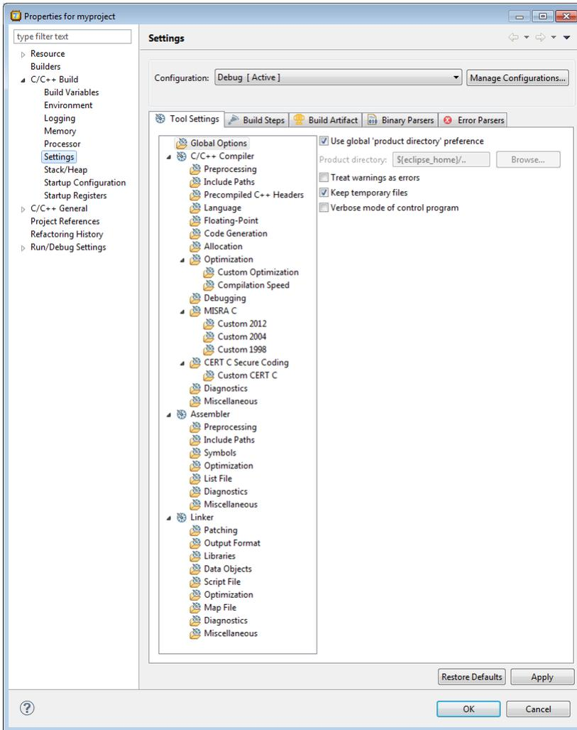
On the **Tool Settings** tab, the options are grouped in Global Options, C/C++ Compiler, Assembler and Linker or Archiver if you are building a library. Note that the options you enter in the Assembler page are not only used for hand-coded assembly files, but also for the assembly files generated by the compiler. In the **Configuration** field, you can choose a configuration for which you want to make changes. Note that this does not make the configuration active.
