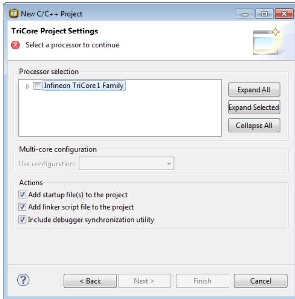
4. Select the target processor for which you want to build the application. For example TC1796B (under AUDO NextGeneration Family). Afterwards you can always change the processor in the **Project » Properties for** dialog.
