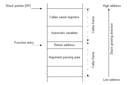
Figure 1.1. System stack layout
