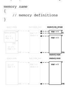
Suppose your embedded system has 56kB of external RAM, named xram, 8 kB of external NVRAM, named my\_nvram and 64kB of external ROM, named xrom (see figure above.) xram and my\_nvram are connected to the bus xdata\_bus and xrom is connected to the bus code\_bus. In LSL this looks like follows:
