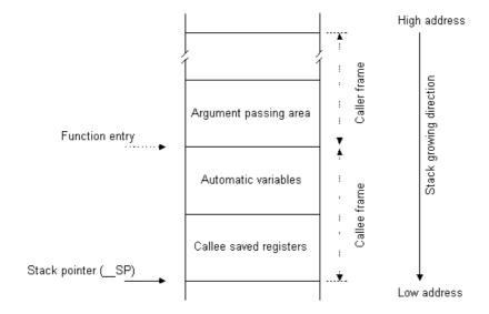
Figure 1.2. Virtual stack layout
